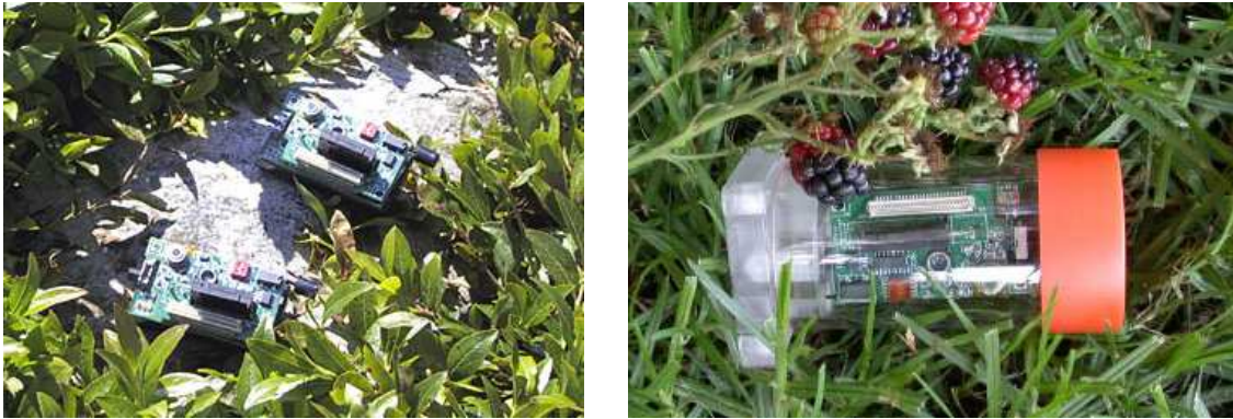
Figure 8: Motes deployed on Great Duck Island
